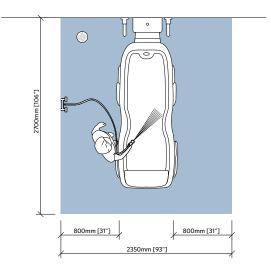
Blue area denotes the required working space to facilitate hygiene and transfer activities while providing adequate access for the resident, equipment and assisting carer.
